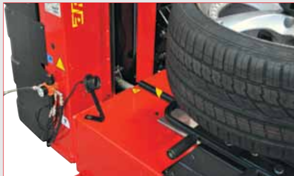
video camera activatable during operations, positioned for a clear view of the lower side of the tyre
