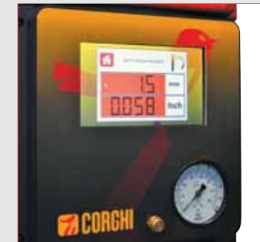
tread depth values: shown with red background to indicate values below minimum limit
